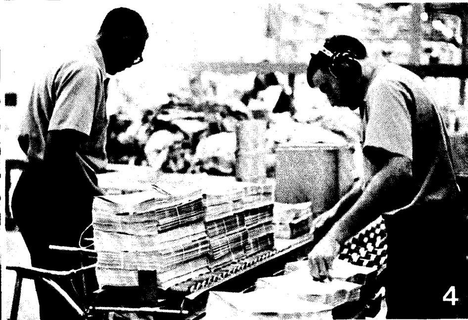
(1-2) The magazines are folded, collated, stapled and trimmed. (3) They are transported to the labeler, where computer-set labels are attached. (4) Then they are tied for mailing.
